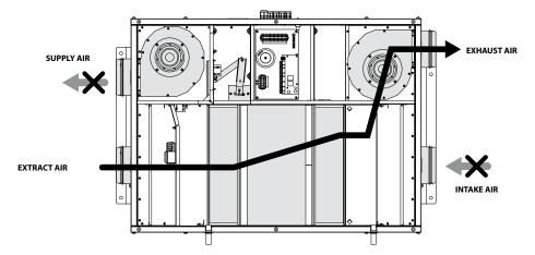
**Summer cooling mode:** the bypass damper is opened, the extract air that is removed from the premises is routed along the bypass duct. The supply air temperature remains the same as the intake air temperature.
