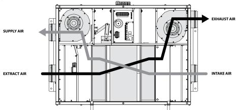
**Freeze protection mode:** this mode is designed for heat exchanger freezing protection and is activated on feedback from the freeze protection temperature sensor in the exhaust air duct. Activation of the freeze protection mode starts when the exhaust air temperature drops down to +3 °C. When the exhaust air temperature exceeds above this temperature point, the unit reverts to the previous operation mode. In the freeze protection mode the supply fan is off, the exhaust fan operates normally.
