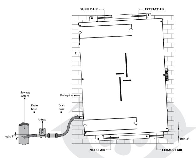
The condensate drain system is designed for use in premises with ambient temperature above 0 °C!
